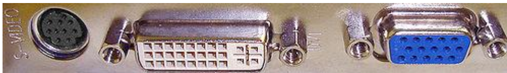
9-pin VIVO for S-Video (TV-out), DVI for HDTV, and DE-15 for VGA outputs.
